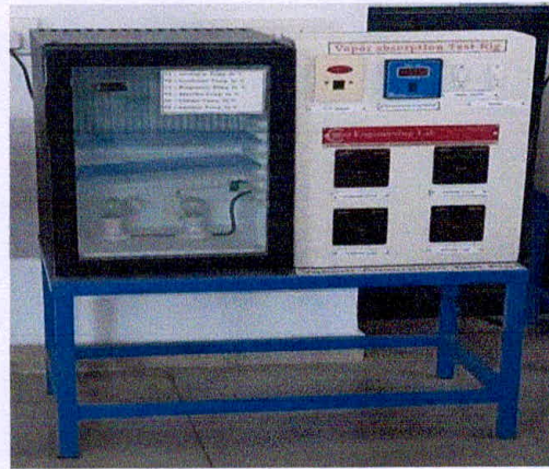
Figure 11.3 Photographic view of Refrigeration Cycle Test Rig.
