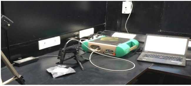
Figure 7 The ASD Fieldspec4 setup for sample spectral reflectance measurement
